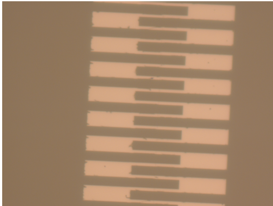
Figure 8: This array shows rips and torn up edges – however it is not as bad as for many arrays. (Optical microscope at 100x)
