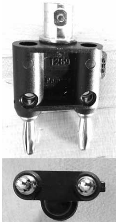
Figure 1: BNC female to dual banana-plug adapter. Note the tab on right labelled “GND”. This indicates which side is electrically connected to the outer conductor of the BNC connector, which is often grounded.
