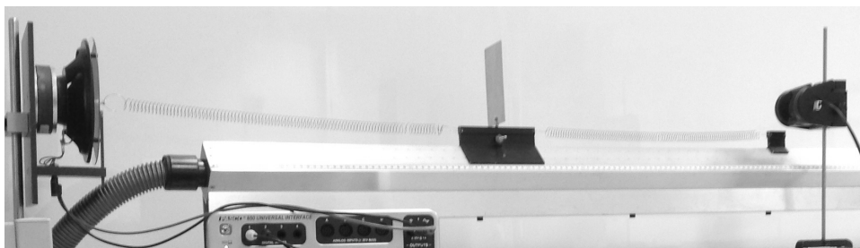
Figure 6: Photo of air track setup with motion sensor and speaker.
