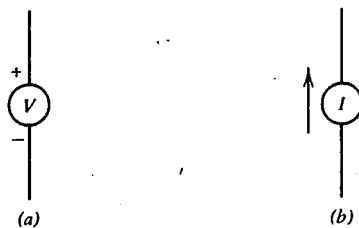
Fig. 1.3 (a) Ideal voltage source. (b) Ideal current source.
