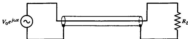
Fig. 5.10 A coaxial transmission line connecting a sinusoidal voltage source to a resistor.
