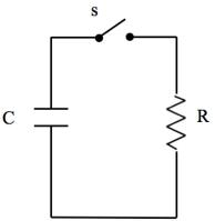
C. What is the current through the resistor at t = 0, the instant when the switch is closed?
