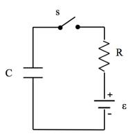
C. At  $t = 2\tau$ , what is the charge on the capacitor, the current through the resistor, and the potential difference across the capacitor?
