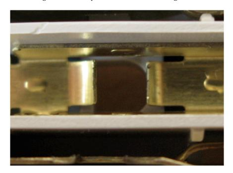
**Used power strip.** Here is an equivalent view of a power strip that's been in use for five years. Things are plugged into it, and removed, every lab. The brass tabs are now tangent to the receptacle opening, and a ground connection is no longer assured.
