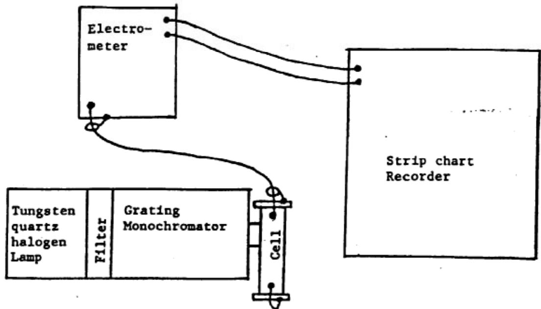
of the experiment the anode is grounded and the photocathode is allowed to charge up to a positive voltage with respect to the anode by photoelectron emission. The cathode voltage is measured using the Keithly electrometer as an extremely high impedance voltmeter. A schematic of the photoelectric battery experiment is shown above.
