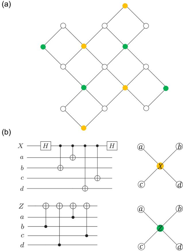
FIG. 3. (a) Architecture of a 17-qubit, distance-3 surface code, introduced in Ref. [21]. Data qubits are denoted by the open circles whereas the X- and Z-syndrome qubits are denoted by orange (light) and green (dark) closed circles, respectively. (b) Standard syndrome-extraction circuits for X and Z syndromes, for the qubit orientations shown on the right. The circuits for the exterior ancillas that have only two neighboring data qubits involve fewer gates, with the same relative ordering.
