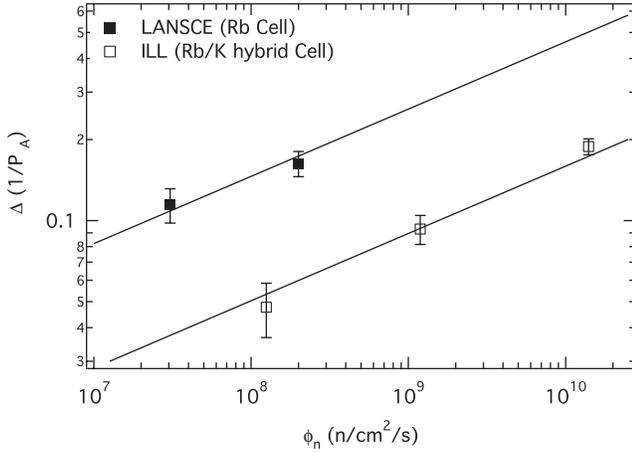
FIG. 4. Neutron-induced change in alkali-metal polarization for the LANSCE Rb cell and the ILL hybrid cell. The solid lines are provided to guide the eye.
