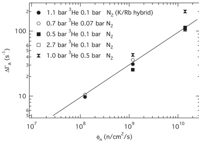
FIG. 5. ILL alkali-metal polarization relaxation results for all cells. Error bars of  $\approx 10\%$  are similar to the size of the symbols. The solid line, provided to guide the eye, is proportional to  $\sqrt{\phi_n}$ .
