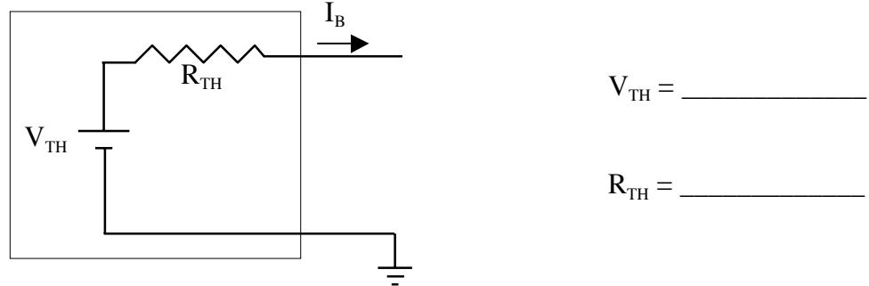
3. Find  $V_B$ . ( $V_B = V_{TH} - I_B R_{TH}$ , from ohm's law.)
