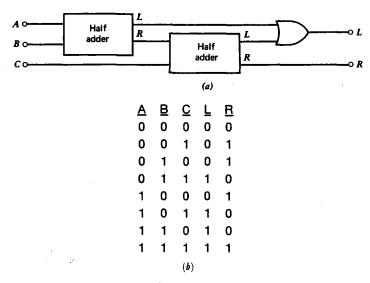
**Fig. 11.8** The full-adder circuit in (a) is described by the truth table in (b).
