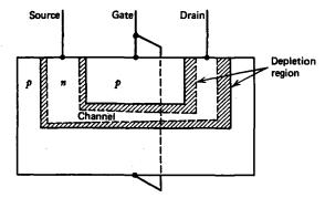
Flg. 7.13 n-channel junction field effect transistor.
