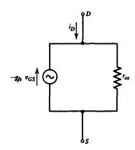
Fig. 7.16 FET linear equivalent circuit.
