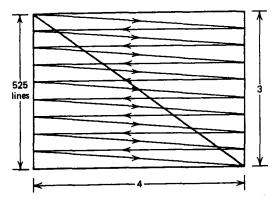
Fig. 12.10 Scan sequence of a television picture.
