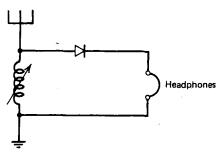
Fig. 12.6 Simple diode receiver.
