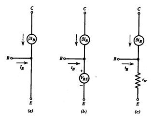
Fig. 8.4 Transistor linear equivalent circuit models. (a) Ideal transistor. (b) de equivalent circuit of ideal germanium or ideal silicon transistor. (c) ac equivalent circuit of real transistor.
