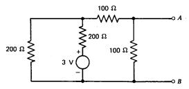
**2.9** For the circuit below, show that the maximum power will be dissipated in R if  $R = R_T$ . This result is extremely useful in the design of circuits that must deliver the maximum possible power.
