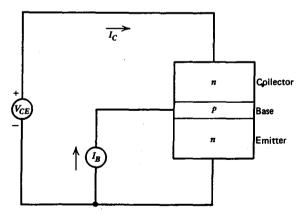
Fig. 8.1 Bipolar npn transistor.
