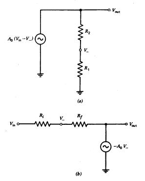
Fig. 9.5 Equivalent circuits for calculating the amplification of the circuits in figure 9.4 for  $A_0$  finite. (a) Voltage feedback. (b) Operational feedback.
