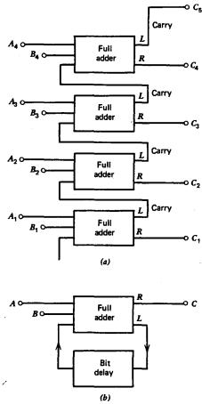
Fig. 11.9 (a) Four-bit parallel adder. (b) Serial adder.
