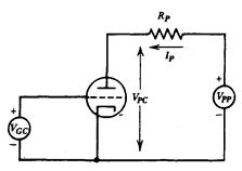
Circuit for determining operating point of a vacuum triode.
