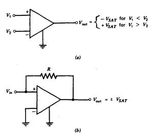
Flg. 9.13 (a) Comparator circuit. (b) Latch circuit.
