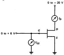
Measure and plot the drain current  $I_D$  versus drain-to-source voltage  $V_{DS}$  for several gate-to-source voltages  $V_{GS}$  in the range 0-6 V.
