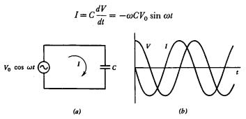
**Fig. 4.2** A sinusoidal voltage source connected to a capacitor (a) produces a current as in (b).
