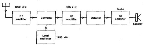
Fig. 12.8 Superheterodyne receiver.
