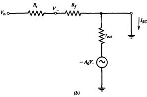
Fig. 9.7 Equivalent circuits for calculating the output resistance of the circuits in figure 9.4. (a) Voltage feedback. (b) Operational feedback.
