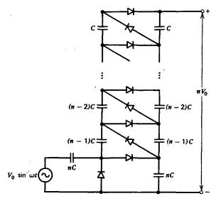
Fig. 6.12 Voltage multiplier circuit.
