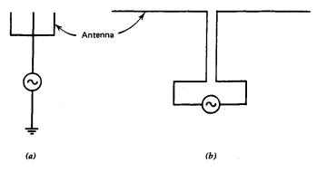
Fig. 12.2 Sinusoidal source connected between: (a) an antenna and ground, (b) two terminals of an antenna.
