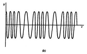
Fig. 12.4 (a) Amplitude modulation. (b) Frequency modulation.
