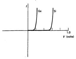
**Fig. 6.4** I versus V characteristic for germanium and silicon diode at room temperature.
