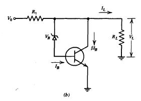
Fig. 8.9 Transistor voltage regulators. (a) Series. (b) Parallel.
