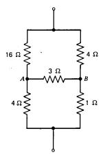
Fig. 1.12 Example of a circuit whose symmetry can be exploited to yield an equivalent resistance of 4  $\Omega$ .
