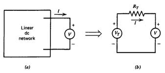
**Fig. 2.5** The current I is the same function of V for circuit (a)and circuit (b) if  $V_T$  and  $R_T$  are chosen appropriately.
