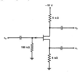
**7.20** In the circuit below, calculate the dc gate-to-source voltage  $V_{GS}$  if the FET is biased such that  $V_{DS} = 0.5 \ V_{DD}$ .
