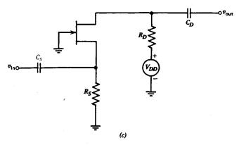
Fig. 7.17 FET amplifier circuits. (a)Common source. (b) Source follower. (c) Grounded gate.
