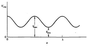
Illustration of standing waves on an improperly terminated transmission line. The VSWR is equal to  $V_{\rm max}/V_{\rm min}$
