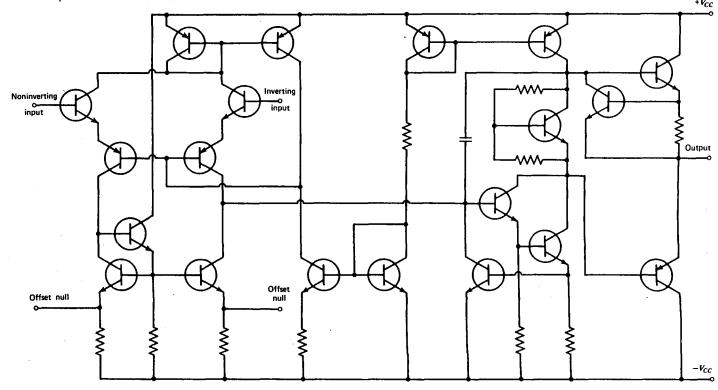
Fig. 9.1 Typical, low-cost, general-purpose operational amplifier.
