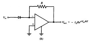
Fig. 9.11 Nonlinear op amp circuits. (a) Logarithmic amplifier. (b) Exponential amplifier.
