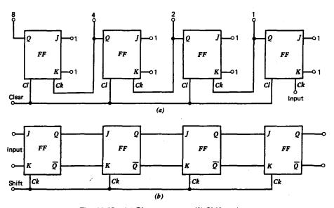
Fig. 11.13 (a) Binary counter. (b) Shift-register.
