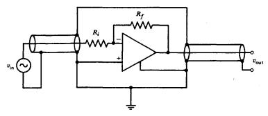
The proper way to isolate an amplifier from unwanted inter-Fig. 9.17 ference.
