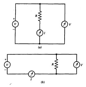
For each case, correct the measured resistance for the finite internal resistance of the meters. Explain under what circumstances each circuit is best for such resistance measurements.
