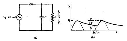
**Fig. 6.9** A rectifier with capacitive filter (a) produces an output as in (b).
