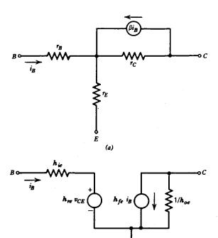
**Fig. 8.5** Four-parameter transistor linear equivalent circuit models. (a) T network equivalent circuit. (b) h parameter equivalent circuit.
