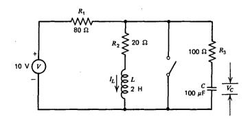
In the circuit below, the current increases linearly with time starting at t=0such that I=0 for t<0 and I=0.01 t for  $t\geq0$ . Find the voltage across the capacitor and the voltage across the inductor if at t = 0 the capacitor is discharged.
