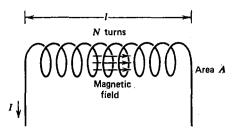
Fig. 3.5 A solenoidal inductor.
