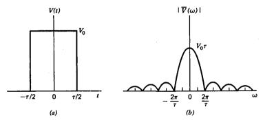
Fig. 5.7 Fourier transform of a square pulse.
