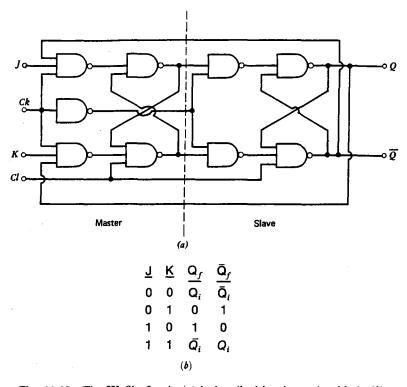
Fig. 11.12 The JK flip-flop in (a) is described by the truth table in (b).
