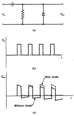
Fig. 6.16 The baseline restoration circuit (a) prevents the baseline of an input signal (b) from drifting downward (c) as the capacitor charges up.
