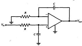
**9.11** Show that the circuit below behaves like a negative resistance (i.e., I decreases as V increases), and calculate the input resistance,  $R_{in} = V/I$ .
