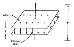
Fig. 3.3 A parallel plate capacitor.
