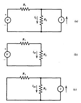
Fig. 2.3 The circuit in (a) can be analyzed using the supposition theorem by considering the simpler circuits in (b) and (c).
