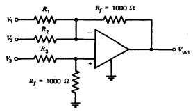
**9.6** Calculate the amplification and the input resistance for the circuit below, assuming the op amp is ideal.
