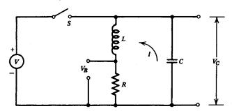
The switch S is a mercury relay that is driven by the 60-Hz voltage from the power line. Verify that it opens and closes every 1/120 s. Adjust the oscilloscope so that it triggers on the opening of the switch. The behavior of the circuit will be studied just after the switch opens, at which time the source is disconnected and the circuit consists only of a series RLC.
