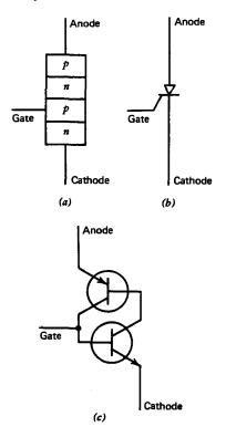
Fig. 10.11 Silicon-controlled rectifier.
