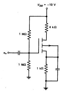
**7.21** Calculate the amplification A, the input resistance  $R_{\rm in}$  and the output resistance  $R_{\rm out}$  for each of the circuits in figure 7.17 in terms of  $g_{fs}$ . Assume  $r_{os} = \infty$  and the capacitors are short circuits for ac.
