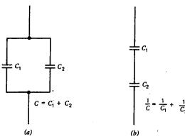
Fig. 3.8 Capacitors in parallel (a) and series (b) add opposite to the way resistors do.
