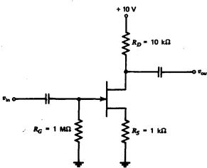
7.19 For the circuit below in which  $g_{fs} = 0.04$  T and  $r_{os} = \infty$ , calculate  $A_1 = v_1/v_{in}$  and  $A_2 = v_2/v_{in}$ , assuming the capacitors are short circuits for ac.
