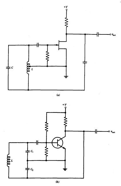
Fig. 10.2 Typical oscillator circuits. (a) Hartley. (b) Colpitts.
