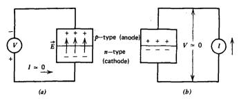
**Fig. 6.3** pn junction diode. (a) Reverse-biased,  $I \simeq 0$ . (b) Forward-biased,  $V \simeq 0$ .
