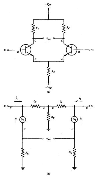
**Fig. 8.11** The difference amplifier in (a) can be analyzed using the linear equivalent circuit in (b).
