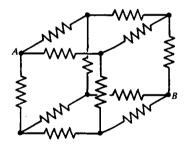
**1.8** For the circuit below, calculate the equivalent resistance between points A and B.
