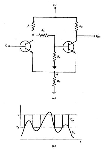
Fig. 10.7 The Schmitt trigger circuit in (a) produces an output (b) that switches between two levels whenever the input voltage crosses the lower of the two levels.
