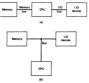
Fig. 11.17 Two possible ways to organize the components of a digital computer. (a) Separate buses. (b) Single bus.
