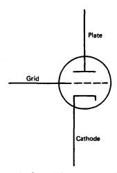
Fig. 7.1 Symbol for a vacuum triode.
