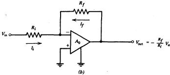
Fig. 9.4 Examples of op amp feedback. (a) Voltage feedback. (b) Operational feedback.
