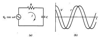
Fig. 4.4 In the sinusoidal series RC circuit in (a), the current leads the voltage by a phase  $\phi = \tan^{-1}(1/\omega RC)$ , as shown in (b).
