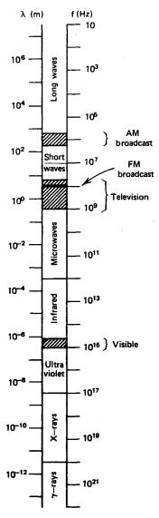
Fig. 12.1 The electromagnetic spectrum.
