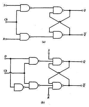
Fig. 11.11 (a) Clocked RS flip-flop. (b) D flip-flop.
