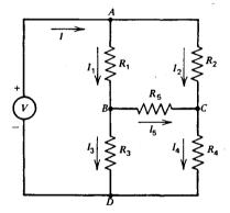
Fig. 2.1 The Wheatstone bridge is an example of a circuit that cannot be analyzed by simple circuit reduction.
