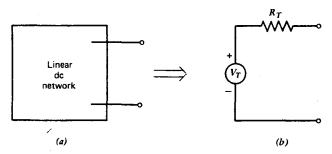
**Fig. 2.4** A linear, two-terminal, dc network (a) can be represented by a voltage source in series with a resistor (b).
