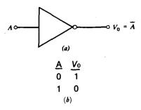
Fig. 11.5 NOT circuit. (a) Symbol. (b) Truth table.
