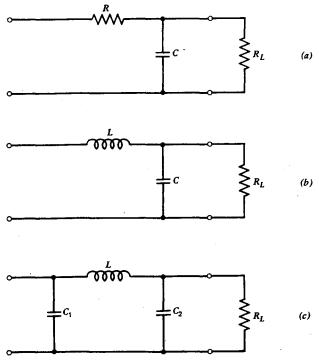
**Fig. 6.10** · Some commonly used filters for rectifier circuits. (a) RC. (b) LC. (c)  $\pi$ -section.
