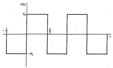
Fig. 5.2 Square wave voltage with period T.
