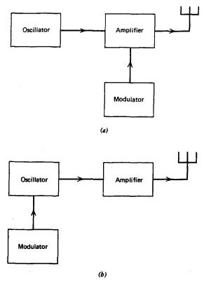
Fig. 12.5 Transmitters. (a) AM. (b) FM.
