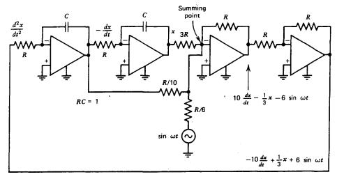
Fig. 9.10 Analog computer circuit for solving the equation
