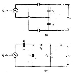
Fig. 6.11 Voltage doubler circuits. (a) Conventional doubler. (b) Charge pump.
