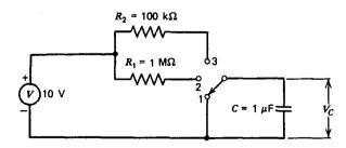
**3.7** In the circuit below, the switch has been open for a long time, and then at t = 0 it is closed. Determine the current I and voltage  $V_3$  just after the switch is closed (t = 0) and after a long time  $(t \to \infty)$ .
