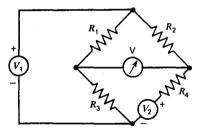
**2.19** Draw the Thevenin equivalent circuit and calculate the values of  $V_T$  and  $R_T$  for the circuit below.
