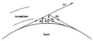
Fig. 12.3 As the frequency is raised or as the ionosphere becomes less dense, a radio wave (a) is reflected at a higher altitude (b) until finally it is not reflected at all (c).
