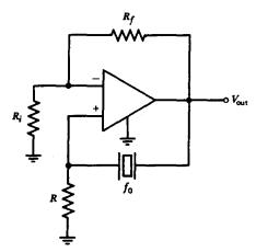
Fig. 10.5 Op-amp crystal oscillator circuit.
