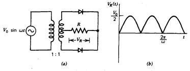
The full-wave rectifier (a) produces an output voltage as in (b).
