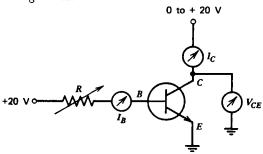
Measure and plot the collector current  $I_C$  versus collector-to-emitter voltage  $V_{CE}$  for several values of base current  $I_B$  in the range  $0-100 \mu A$ .
