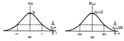
Fig. 5.6 The Fourier transform of a gaussian (a) is another gaussian (b) whose width is inversely proportional to the width of the first.
