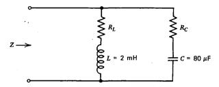
**4.9** For the circuit below calculate the Thevenin equivalent voltage and the Thevenin equivalent impedance. Show how the Thevenin equivalent circuit could be constructed using individual circuit elements (resistors, inductors, etc.) in series, and indicate the required values.
