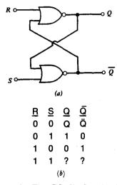
Fig. 11.10 The RS flip-flop in (a) is described by the truth table in (b).
