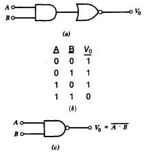
Fig. 11.4 (a) NAND circuit. (b) Truth table. (c) Symbol.
