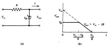
**Fig. 6.19** The Zener diode regulator in (a) produces an input voltage as in (b) that is constant so long as the output current is small.
