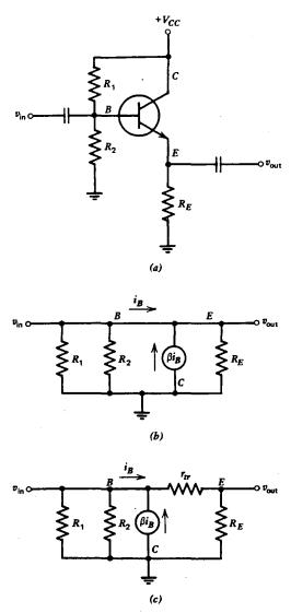
**Fig. 8.7** The emitter follower circuit in (a) can be analyzed using the linear equivalent circuit in (b) if the transistor is ideal, or using the more realistic model in (c) if more accurate results are required.
