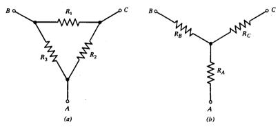
Fig. 2.10 Representations of a three-terminal, dc, passive network. (a)  $\Delta$ -connection. (b)  $\Upsilon$ -connection.
