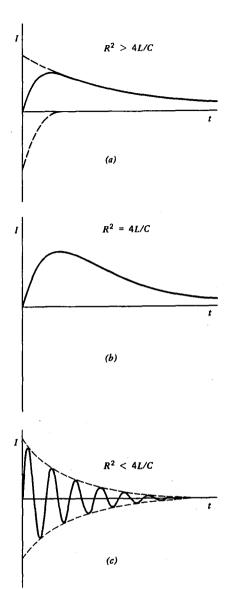
Fig. 3.12 Current versus time for a series RLC circuit. (a) Overdamped. Critically damped. (c) Underdamped.
