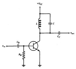
Fig. 8.15 Class C amplifier with resonant output circuit.
