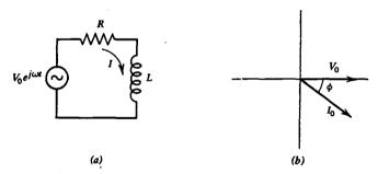
Fig. 4.6 The circuit in (a) has a phasor diagram as in (b) where  $\phi$  $= \tan^{-1} \left( -\omega L/R \right).$
