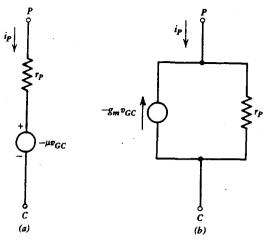
Vacuum tube linear equivalent circuits. (a) Thevenin. (b) Norton.
