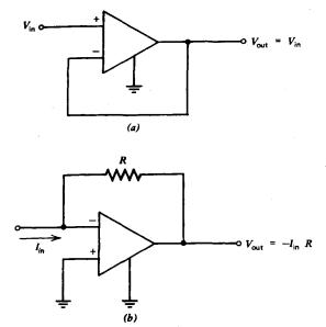
Fig. 9.8 Special cases of feedback amplifiers. (a) Voltage follower. (b) Current-to-voltage converter.
