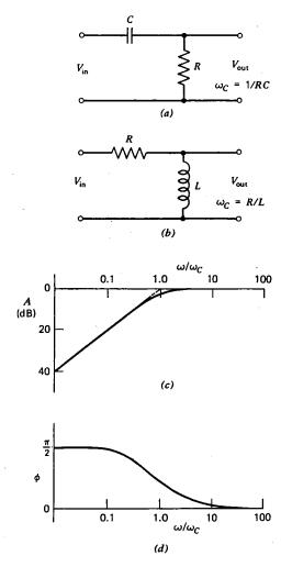
Fig. 4.9 The high-pass filters in (a) and (b)produce an attenuation (c) and phase (d) that vary with frequency.
