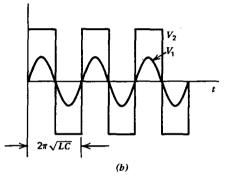
Fig. 10.1 The op amp oscillator circuit in (a) produces a sinusoidal and a square wave output as shown in (b).
