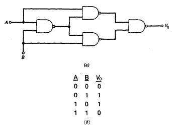
Fig. 11.16 The exclusive-OR circuit in (a) whose truth table is in (b) is an example of controlling the operation of a circuit by means of an instruction.
