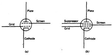
Fig. 7.11 Multigrid tubes. (a) Tetrode. (b) Pentode.
