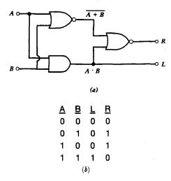
Fig. 11.7 The half-adder circuit in (a) is described by the truth table in (b).
