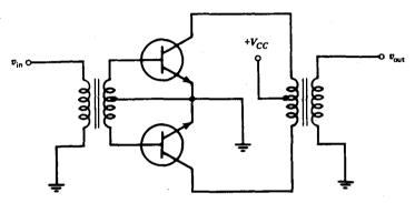
Fig. 8.13 A push-pull amplifier uses two matched transistors biased to cutoff (class B).
