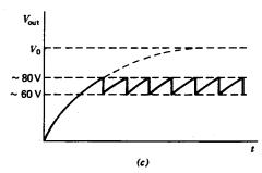
**Fig. 10.9** The neon bulb (a), because of its negative resistance characteristic, can be used in a relaxation oscillator circuit (b) to produce a sawtooth output voltage (c).
