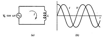
Fig. 4.3 A sinusoidal voltage source connected to an inductor (a) produces a current as in (b).
