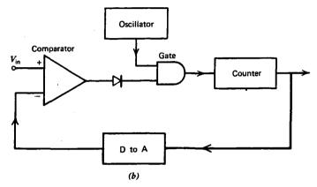
Fig. 11.14 (a) Digital-to-analog converter. (b) Analog-to-digital converter.
