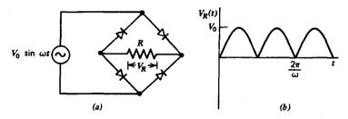
**Fig. 6.8** The bridge rectifier (a) produces an output voltage as in (b).
