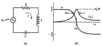
The series RLC circuit in (a) exhibits resonant behavior as shown Fig. 4.7 in (b).
