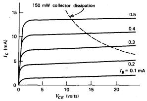
Fig. 8.3 Typical bipolar transistor collector characteristics.
