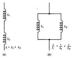
**Fig. 3.7** Inductors in series (a) and parallel (b)add just as resistors do.
