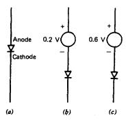
Fia. 6.5 (a) Ideal diode. (b) Germanium diode. (c) Silicon diode.
