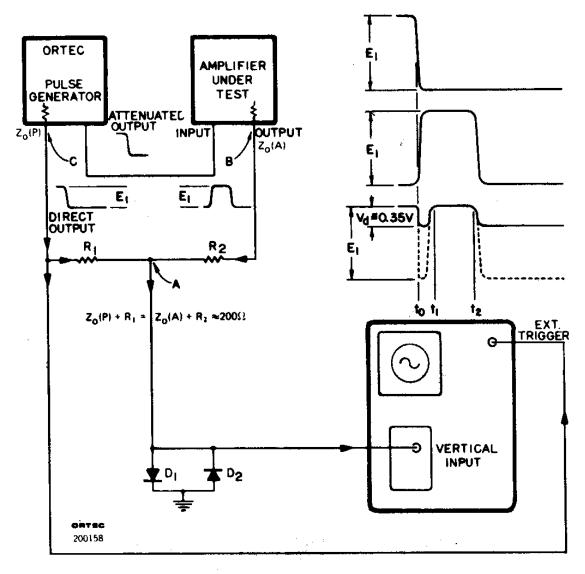
Fig. 4.5. Measuring Linearity by the Null-Balance Method.
