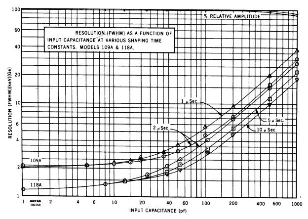
Fig. 4.2. Resolution Spread vs. External Input Capacity.
