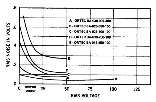
Fig. 4.4. Amplifier and Detector Noise vs. Bias Voltage.
