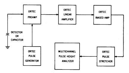
Fig. 4.3. Measuring Resolution with a Pulse Height Analyzer.
