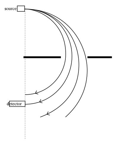
The particles of different momenta will pass through different focus points. By using a small source and a small detector only those in a small range from p to p + dp will be accepted.
