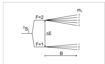
Fig. 2 Schematic representation of Zeeman levels in the ground state of  ${}^{87}$ Rb Hyperfine splitting  $\Delta E$  and Zeeman splitting are not drawn to scale.
