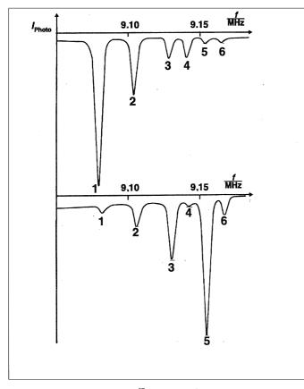
Fig. 5: Absorption spectrum  $^{87}\text{Rb}$  with  $\sigma^+$  light (top) and  $\sigma^-$  light (bottom). For identification of the absorption lines see Table 2.
