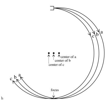
1. Variation of Angle. Consider several electrons emitted with the same momenta but at slightly different angles. Each particle will follow a circular path with a slightly different center point.
