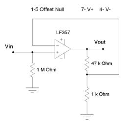
Clip the component leads short and bend them so the component bodies lie flat against the breadboard – this minimizes stray capacitances. Use a single bus on the socket for all the grounds (probably the inner strip below the op-amp). It is a good idea to put  $0.1 \ \mu F$ capacitors from the +15V and the -15V supply pins of each op-amp to ground to bypass the power supply.
