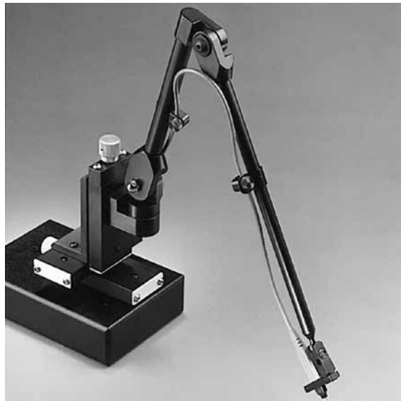
Figure 2.11. Example of a probing station designed for probing small geometry devices such as hybrid circuits and ICs.
