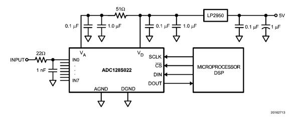
FIGURE 8. Typical Application Circuit
