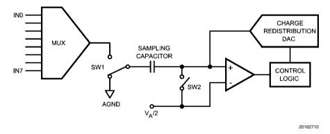
FIGURE 5. ADC128S022 in Hold Mode
