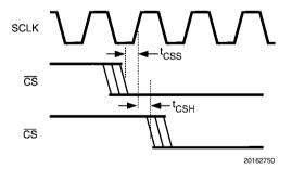
FIGURE 3. SCLK and  $\overline{\text{CS}}$  Timing Parameters
