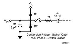
FIGURE 7. Equivalent Input Circuit
