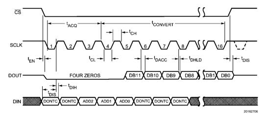
FIGURE 2. ADC128S022 Serial Timing Diagram
