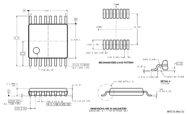
16-Lead TSSOP Order Number ADC128S022CIMT, ADC128S022CIMTX NS Package Number MTC16
