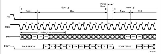
FIGURE 1. ADC128S022 Operational Timing Diagram
