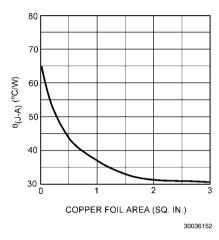
FIGURE 5. θ<sub>JA</sub> vs Copper Area for TO-263 Package
