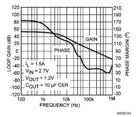
FIGURE 2. Gain-Bandwidth Plot for 1.5A Load
