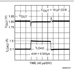
**FIGURE 4. Load Transient Response**
