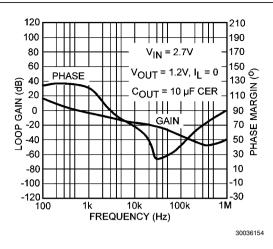
FIGURE 3. Gain-Bandwidth Plot for No Load
