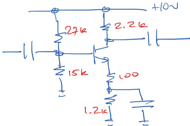
$$\underline{\underline{A}} \quad V_B \approx 10V \times \frac{15k}{15k+27k} = 3.6V$$
