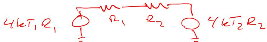
$$S_I = \frac{2k(T_1 R_1 + T_2 R_2)}{(R_1 + R_2)^2}$$
