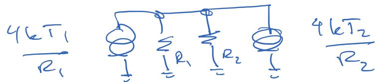
$$\begin{aligned} S_v &= 4k \left[ \frac{T_1}{R_1} + \frac{T_2}{R_2} \right] (R_1 \parallel R_2)^2 \\ &= 2k \left[ T_1 R_2 + T_2 R_1 \right] \left[ \frac{R_1 R_2}{(R_1 + R_2)^2} \right] \end{aligned}$$
