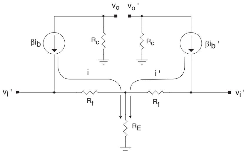
We can get 4 equations by applying ohm's law to this equivalent circuit.
