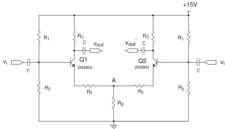
Figure 1: Schematic of the Difference Amplifier
