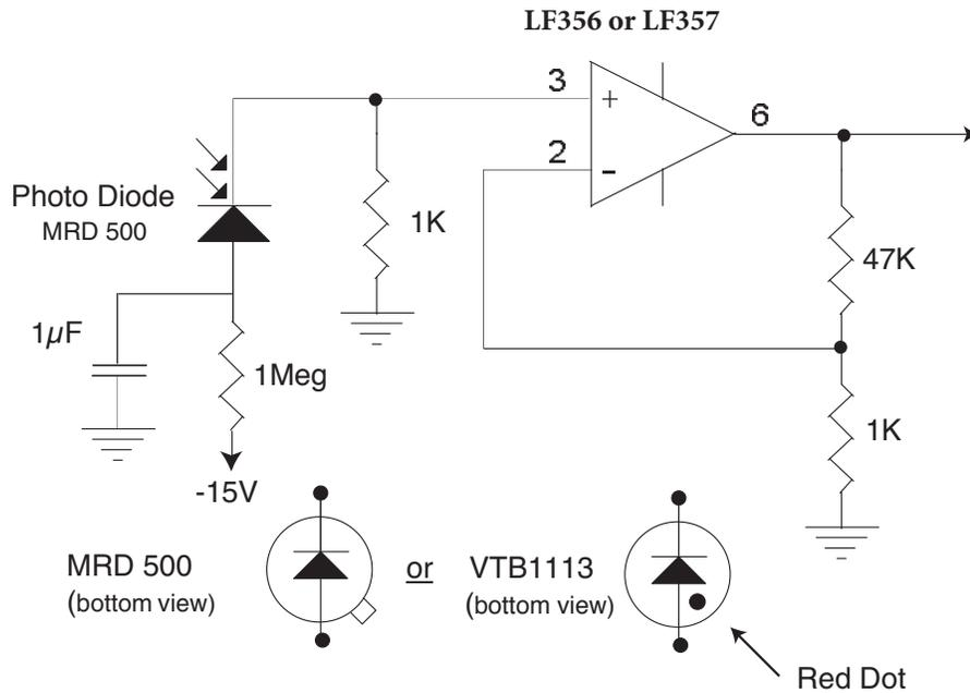
Put a  $\sim 25$  mm piece of black tubing over the end of your photodiode to limit the amount of background light. Bend the leads so it is aimed nearly horizontally at the left end of your breadboard, pointing it a part of the room that is not too bright (set up a dark screen, if necessary). Put a red LED in series with a 100 ohm resistor (available as a packaged unit in a BNC connector) and connect it to the pulse generator input as shown below.
