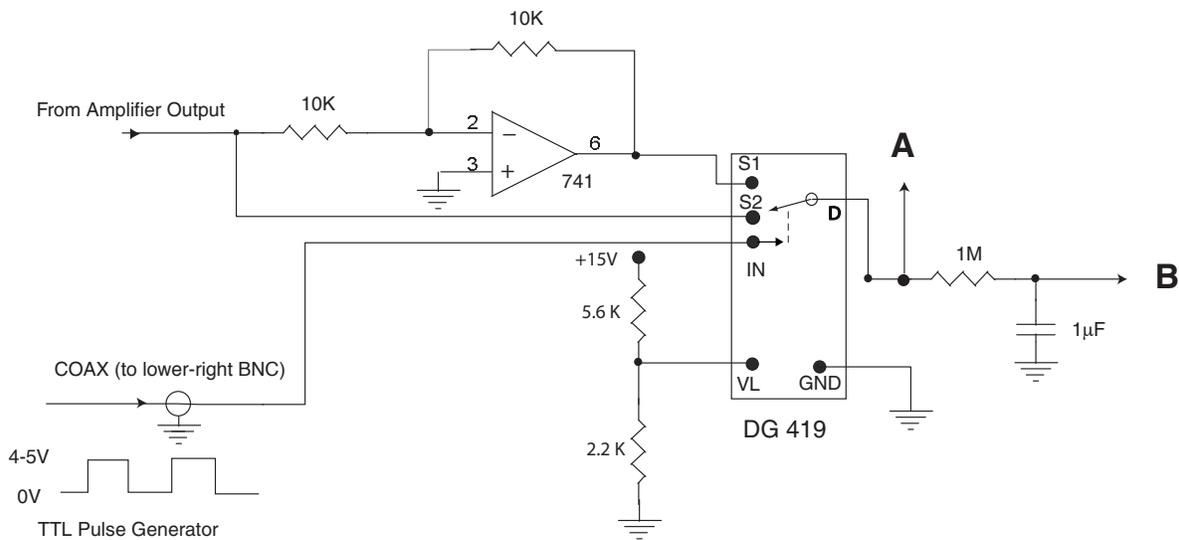
Set the pulse generator to give a 5 V square wave output at a frequency near  $f_0$ . Replace the 1 M resistor at the previous lab LF356/7 amplifier input with a 1 K and add a photodiode as shown below:
