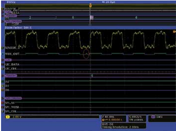
Figure 6. Wave Inspector® reveals a glitch on the MUX_OUT signal.
