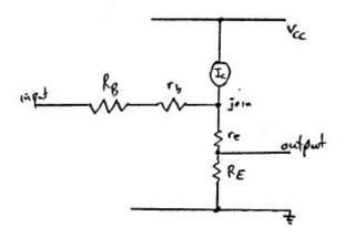
We concern ourselves only with the current and voltage increments so can ignore the +0.7 volt battery. Define the voltage on the point below the current generator at the join of the 3 lines as  $\Delta V_{join}$
