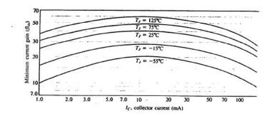
Even though  $\beta$  does not change much with voltage and current, in any given transistor, the variation in  $\beta$  due to temperature and manufacturing is significant. The variation due to manufacturing, can be minimized by selecting transistors with particular values of  $\beta$ .
