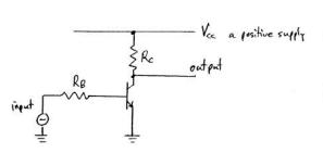
Variations  $\Delta V_{input}$  in the base input voltage will cause variations in the emitter current through  $r_b$ . The transistor can be replaced for calculation purposes by the transistor model as in the next diagram. If, as usual,  $r_e$  is small, then
