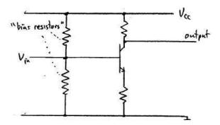
A simple way of "biassing" the AC common emitter is to add two resistances with resistances higher than the emitter resistor so that the "drain current" draining down through both "bias resistors" satisfies two requirements.
