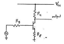
This has 3 resistors as shown  $R_B$ ,  $R_E$  and  $R_C$  attached to the base, emitter and collector. The top "rail" is attached to a positive power supply (perhaps +10 Volt). The lower "rail" is the ground.
