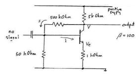
The circuit is similar to the previous common emitter amplifier but the biasing structure has been changed to include some negative feedback from output signal on the collector. As a result, this circuit gives an amplification which is more predictable in spite of variations in the  $\beta$  of the transistor.
