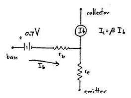
We insert a "Current Generator" in the collector to cause a current  $I_C = \beta I_b$ .
