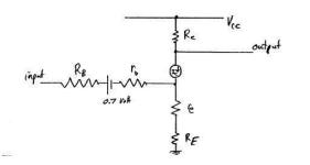
We concern ourselves only with the current and voltage increments so can ignore the +0.7 volt battery. Define the voltage on the point below the current generator at the join of the 3 lines as  $\Delta V_{join}$  We can obtain 2 equations.
