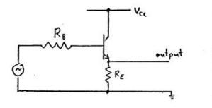
This has 2 resistors as shown  $R_B$  and  $R_E$  attached to the base and emitter. The top "rail" is attached to a positive power supply (perhaps +10 Volt). The lower "rail" is the ground.
