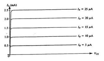
Although the following curves are not usually shown in specifications, the following shows  $I_{Collector}$  and  $I_{Base}$  curves for equispaced collector voltages.
