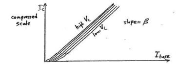
6. Thus  $\alpha$  and particularly  $\beta$  are useful parameters because they are nearly constant for any given bipolar junction transistor over a range of working voltages and currents.
