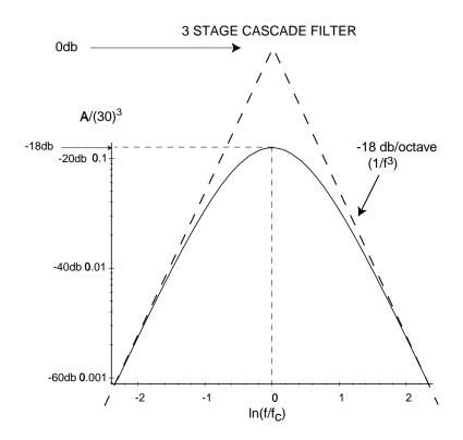
Question 11 What is the gain of the three stage amplifier at f=60 Hz?
