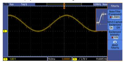
Figure 3: Example of NOISY SINE with Peak Detect mode (FilterVu)
