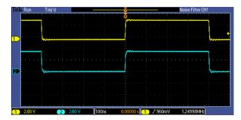
d. Both channel 1 and channel 2 are DC coupled (by default) and are the same. What will happen to the displayed channel 1 signal (yellow waveform) if AC coupling is selected for channel 1?
