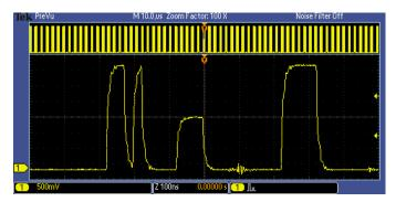
Figure 2: Long waveform record acquisition with a runt trigger event
