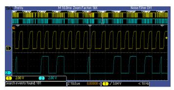
Figure 3: Wave Inspector automatic search for glitches.
