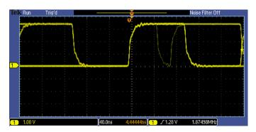
d. Based on the screen shot in step c, set up the oscilloscope's trigger to capture the anomaly. Write down your trigger type and trigger parameters. (Hint: Review your answer to Exercise #1 in the "Capturing Digital Anomalies" section.)
