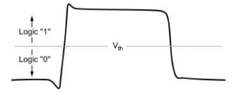
Figure 5: Logic Threshold
