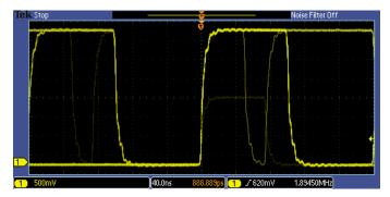
Figure 1: Intensity-graded display showing infrequent transients
