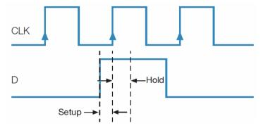
Figure 7: Setup and Hold Time
