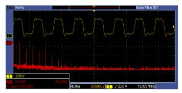
Figure 4: FFT plot of a pulse stream.
