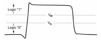
Figure 6: Dual Threshold Logic
