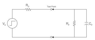
Figure 7: Simplified circuit diagram using Thevenin equivalent of DUT.
