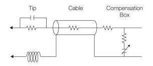
Figure 11: Passive Probe Schematic.
