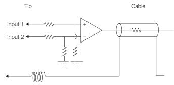
Figure 15: Differential Probe Schematic.
