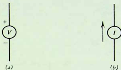
Fig. 1.3 (a) Ideal voltage source. (b) Ideal current source.
