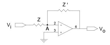
Assume that point A is a virtual ground (*i.e.*  $V_{-} = V_{+}$ ), and that  $I_{i} = 0$ , and prove the general result that
