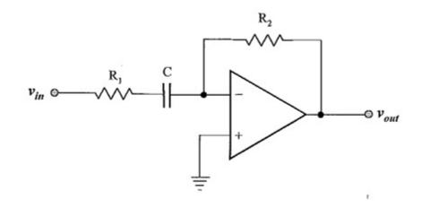
b) Show that, when  $R_1 \ll 1/\omega C$ ,  $(\Rightarrow \omega \ll 1/R_1 C)$ , the circuit works as a differentiator. Find  $V_{out}$ . when  $R_1 \gg 1/\omega C$ ,  $(\Rightarrow \omega \gg 1/R_1 C)$ . 2) With an op-amp, one can also construct a difference amplifier.
