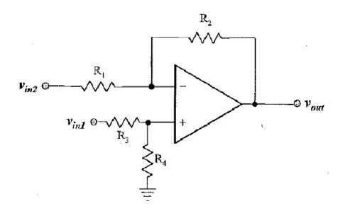
b) Show that when  $R_4/R_3 = R_2/R_1$ , the circuit works as a difference amplifier. What is the voltage gain for a difference input? (Differential gain  $V_{out}/(V_{in1} - V_{in2})$  What is the voltage gain for a common-mode input? (Common mode gain  $V_{out}/[(V_{in1} - V_{in2})/2]$ ).
