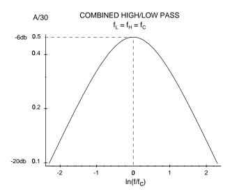
Therefore, the maximum gain of the stage is  $1/2(R_f/R_1) = 15$  at  $f_0$ , and drops off  $\propto f$  for  $f \ll f_0$  and as 1/f for  $f \gg f_0$  – both 6 *db per octave*. What is  $f_0$  for the given component values?
