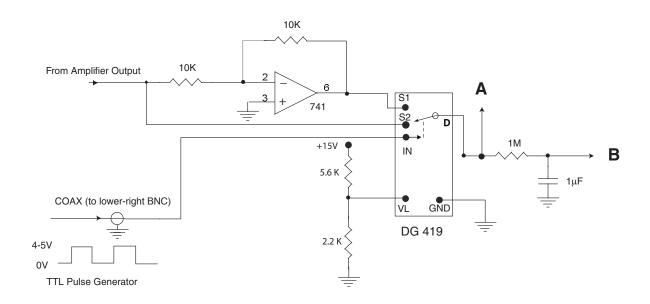
Set the pulse generator to give a 5 V square wave output at a frequency near  $f_0$ . Replace the 1 M resistor at the previous lab LF356/7 amplifier input with a 1 K and add a photodiode as shown below:
