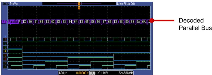
4. In the previous steps, the oscilloscope is triggering on the rising edge of the D0 digital signal. (Autoset sets the trigger source to the lowest active channel.) The oscilloscope can also be set to trigger on parallel bus values.
