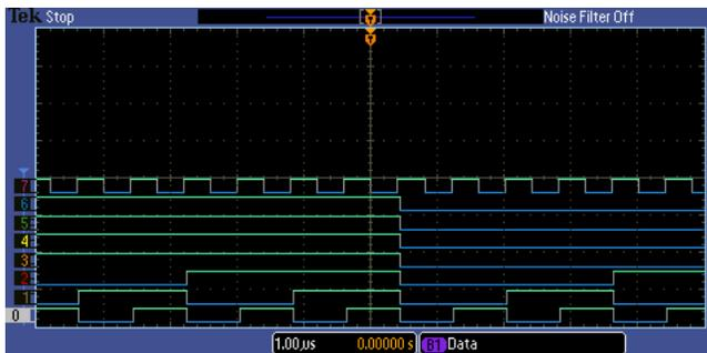
**This display shows triggering on 7F hex or 0111 1111 binary. Notice that the trigger point is at the first point where the MSB goes low and the rest of the bits are all high.**
