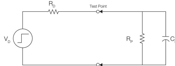
*Simplified circuit diagram using Thevenin equivalent of the DUT*
