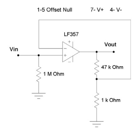
Clip the component leads short and bend them so the component bodies lie flat against the breadboard – this minimizes stray capacitances. Use a single bus on the socket for all the grounds (probably the inner strip below the op-amp). It is a good idea to put  $0.1 \ \mu F$ capacitors from the +15V and the -15V supply pins of each op-amp to ground to bypass the power supply.
