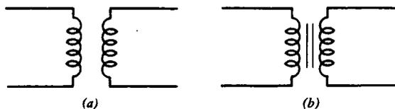
**Fig. 4.12** Symbols for ideal transformer. (a) Air core. (b) Iron core.
