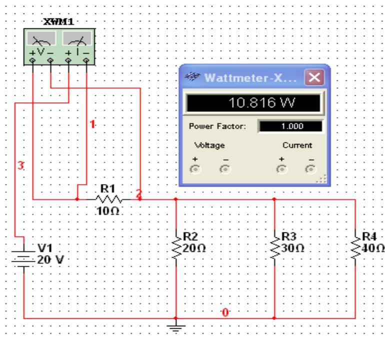
Figure 15: Wattmeter Connection
