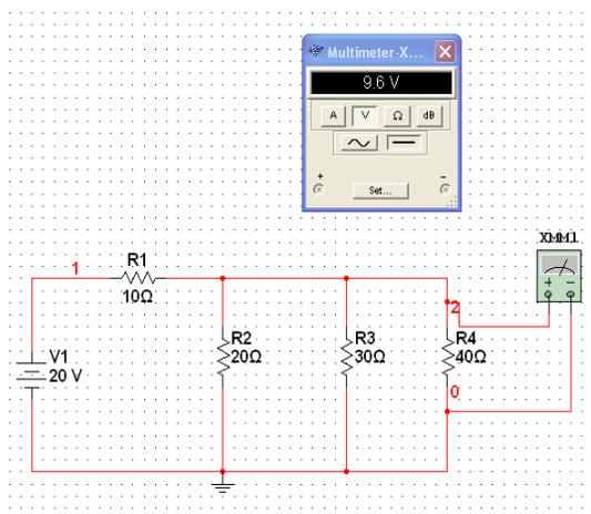
**Figure 12:** Measure Voltage
