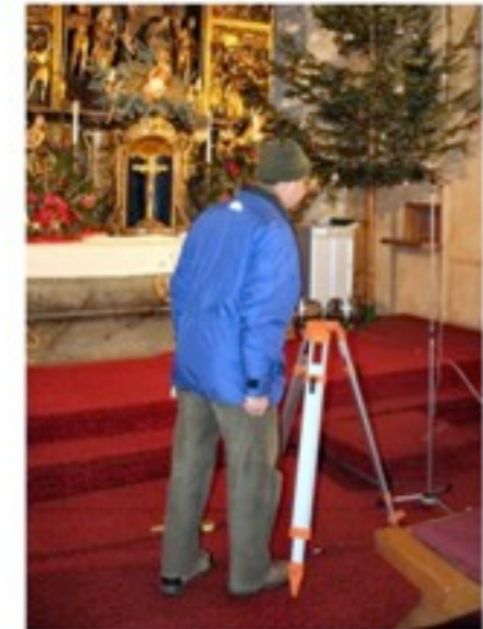
Fig. 3. Vertical gravity gradient measurement; the CG-5 gravimeter is placed on a tripod in the upper position (1 m elevation difference).
