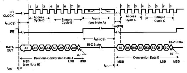
NOTES: A. The conversion cycle, which requires 36 internal system clock periods (17 μs maximum), is initiated with the eighth I/O clock pulse trailing edge after CS goes low for the channel whose address exists in memory at the time.
