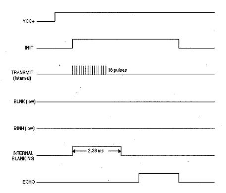
The signal that indicates that an object was found some distance away is from the return of the 16 pulses of TRANSMIT, which is indicated by ECHO. These are all TTL signals naturally. This element draws only 50 mA, so is suitable as a remote sensor.
