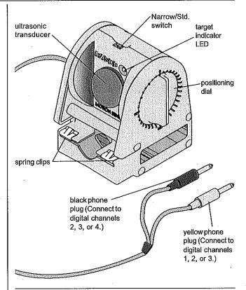
Important Operating Note: When operating in the Std. mode, it may be necessary to tilt the transducer up 5-10 degrees for best performance, as shown.
