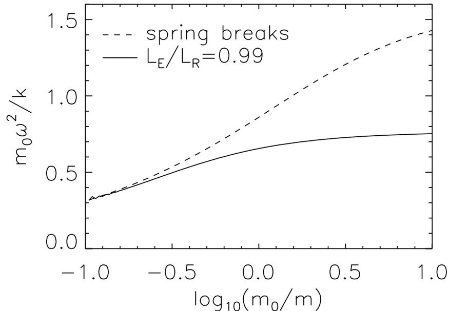
FIG. 4: Comparison of estimate and exact calculation. As  $\omega$  is increased for a given  $m_0/m$ , the estimate increasingly underestimates the actual length of the spring. This underestimation reaches 1% at the solid line, and grows infinite at the dashed line.
