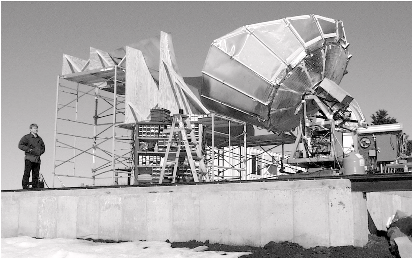
Ph.D. candidate Slade Klawikowski is in charge as the COMPASS telescope searches for primordial polarization in the microwave background radiation at UW's Pine Bluff Observatory.
