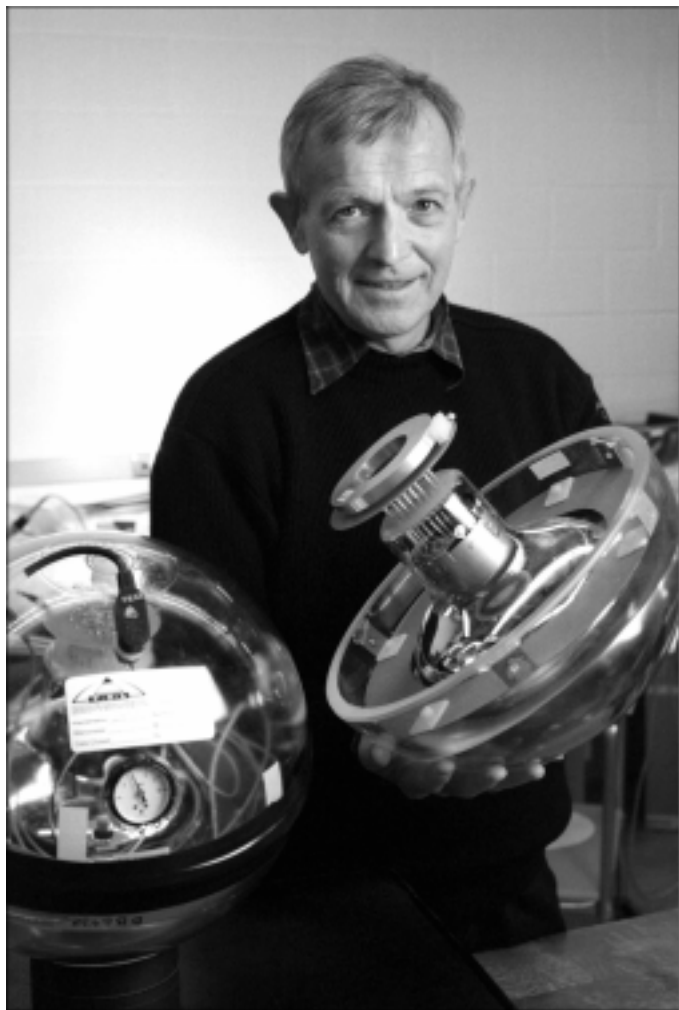
Francis Halzen, a UW-Madison professor who helped develop AMANDA, shows the inside of one of the 422 basketball-sized glass orbs, called photomultiplier tubes, used to catch the fleeting signals left by high-energy neutrinos.
