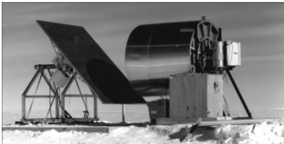
"Big Plate" at Dome C. A 1.5 m diameter reflector telescope points at a large steerable mirror, which sweeps the beam across the sky to make a map of the 2.7 K cosmic microwave background radiation. At the far right, behind the telescope, is a cryostat that cools the detectors to 300 mK.
