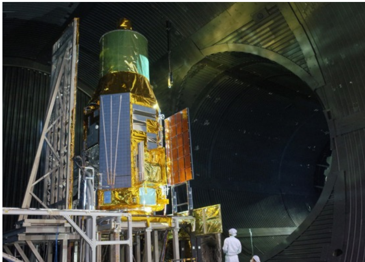
Completed spacecraft in the thermal-vacuum test chamber
