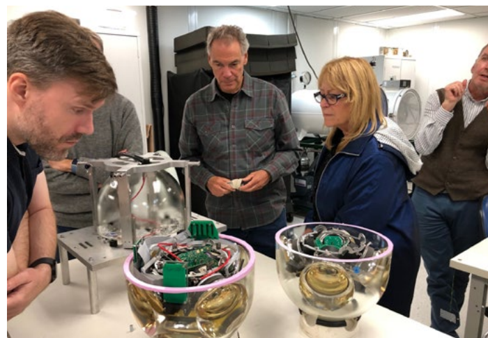
Prof. Albrecht Karle (far right) and BoV members inspect a Digital Optical Module (DOM) under development for the Second Generation of the IceCube neutrino observatory being fabricated at PSL.
