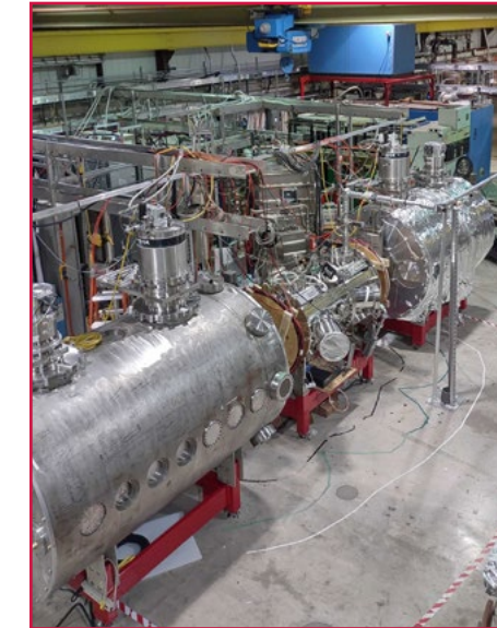
Realta Fusion is developing fusion technology that uses a magnetic mirror to control plasma. Its design is based on the WHAM experimental device developed at UW–Madison, pictured here.
