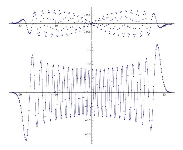
FIG. 2. The lower graph shows the analytical Airy function solution to the Schrödinger equation for the n = 50 state of a linear potential, compared to the Numerov method eigenfunction (dots). The upper graph shows the difference between the analytical and Numerov wave functions.
